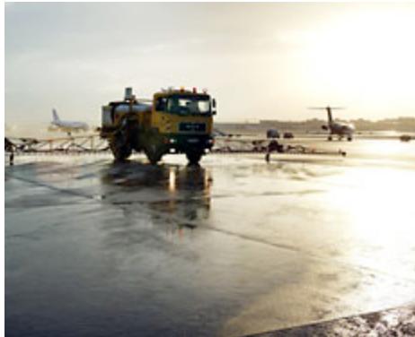
Runway de-icing with special formic acid salts: Ice and snow are melted highly effective, ensuring better ground grip of the aircraft wheels. In sharp contrast to ordinary de-icing salt there are practically no corrosive effects. And: The acid is biodegradable
